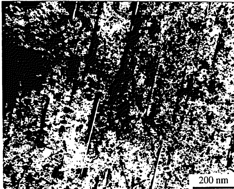
Figure 8b: g/3g weak-beam micrographs of fatigued samples with large SDAS
