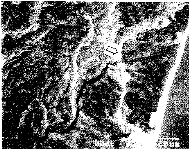
Figure 5.25 A micrograph showing a chemical notch (arrow) on a crack-initiation site of an API-S135 fatigue fractured in deaerated drilling fluid ( T = 93.3 °C, \Delta S/2 = 255.8 MPa, R = 0.1 , f = 2 Hz).
