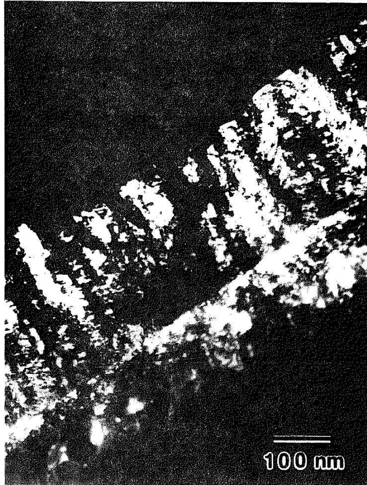
Figure 36: XTEM dark field micrograph, Nickel oxide/sapphire, RF series IIC
