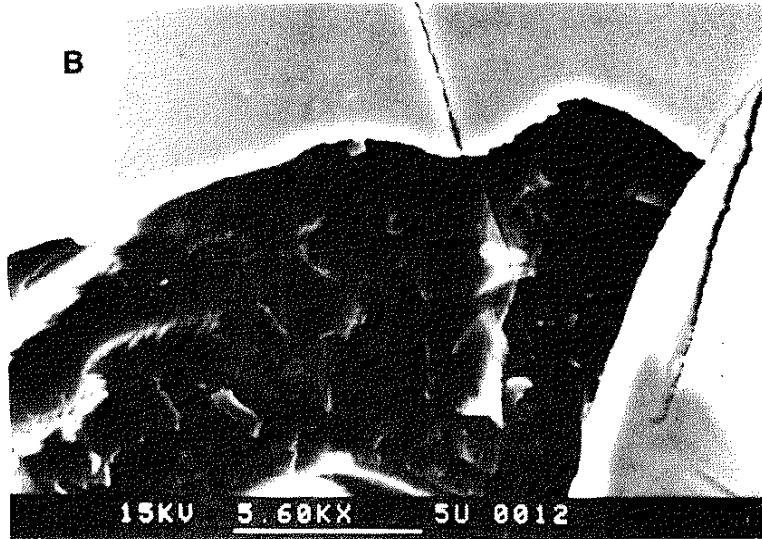
Figure 25: SEM micrographs of Vickers microhardness indents, Nickel/sapphire, RF series IIA, 700 g load A) Low magnification B) High magnification
