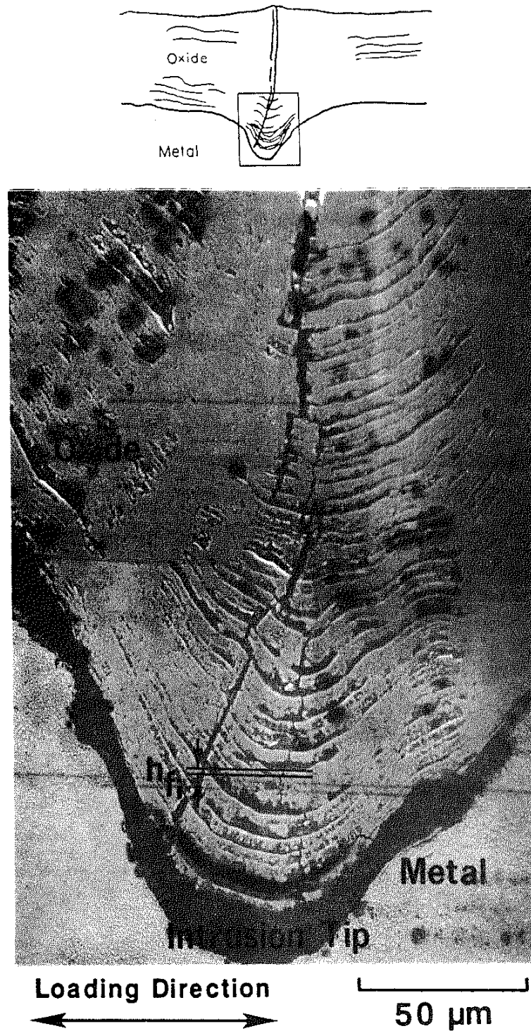
Figure 10 SEM microphotograph illustrating the multi-layer oxide and an h_f measurement (Out-of-phase TMF, T = 500\text{-}600^\circ\text{C} , \Delta\varepsilon_{\text{mech}} = 0.0017 , \dot{\varepsilon} \approx 0.0001 \text{ sec}^{-1} ).
