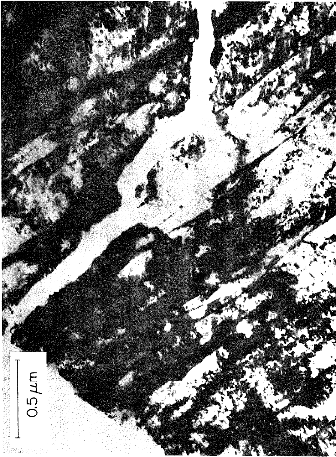
Figure 10 Dislocated lath structure from a laser alloy with 12.5 percent Cr and 1.5 percent Ni that showed BCC single-crystal diffraction pattern and no orientation relationships between laths.
