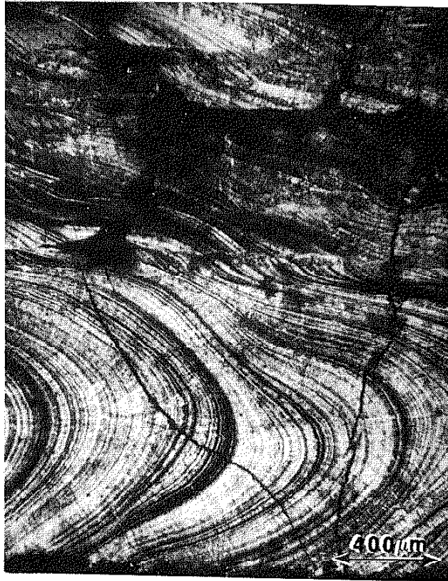
Figure 19. Surface appearance and cracks of laser processed gray iron (2 kW, 2 RPM, 3 overlaps). 50x
