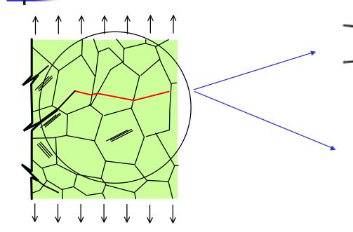
Stage II fatigue cracks much larger than the grain size and are thus sensitive only to large scale microstructural features - texture, global residual stresses, etc.
