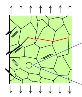
Cyclic slip occurs within a grain and therefore operates on an atomic scale and are thus is controlled by features seen at that scale.
