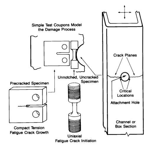
The fatigue life of an engineering component consists of two main life periods:
