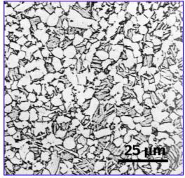
Ti6Al4V annealed at 973 °K in a region having both  $\alpha$  and  $\beta$  equi-axed grains. Upon slow cooling get? plus Widmanstatten  $\alpha$ .
