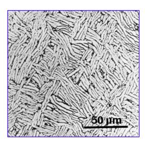
Ti6Al4V annealed at T>1278? °K in the ß field. Upon cooling, get Widmanstatten or basket weave as  $\beta$  ->  $\alpha$  by diffusion.
