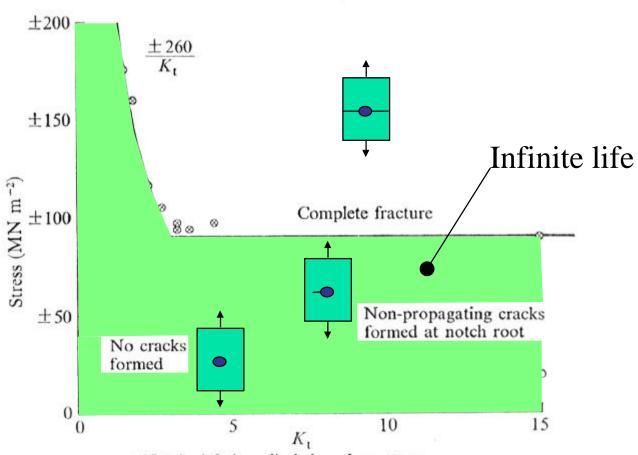
Sharp notches may nucleate cracks but the remote stress may not be large enough to allow the crack to leave the notch stress field.
