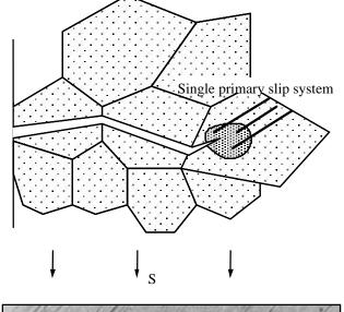
Stage I fatigue cracks are the size of the grains and are thus controlled by features seen at that scale: grain boundaries, mean stresses, environment.
