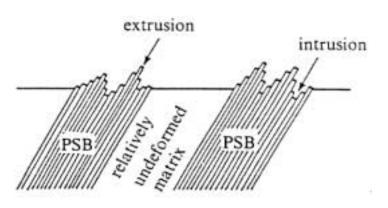
Fatigue crack initiation at an inclusion Cyclic slip steps (PSB)
