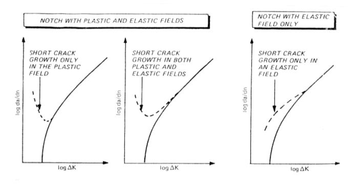
Here the  $\Delta K$  is the remote stress intensity factor based on remote stresses....
