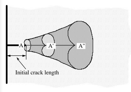
A, A', A" Crack tip positions
