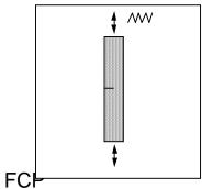
Cracked specimen (Kt > 5) - in the absence of tensile residuals and for near conditions, large grain size preferred
