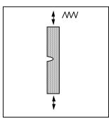
Notched Specimen (Kt ≈ 2) - at long lives initiation and crack growth equally important. Avoid high tensile residuals therefore use lower strength materials
