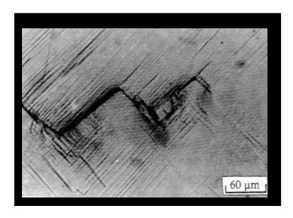
Stage I crack growth ( $r_c \le d$ ) is strongly affected by slip characteristics, microstructure dimensions, stress level, extent of near tip plasticity
