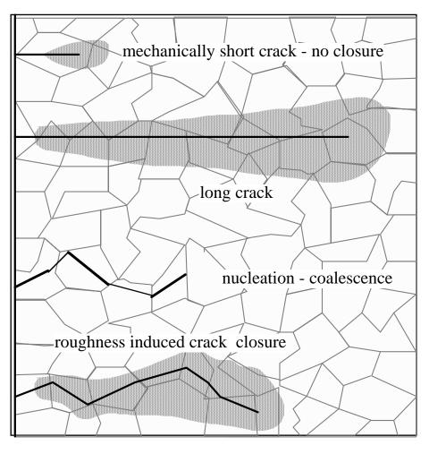
How fatigue cracks grow and particularly the 3-D aspects of fatigue crack growth is not fully understood.
