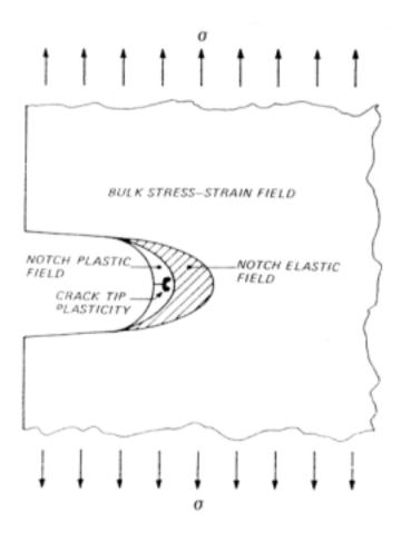
Cracks growing from notches don't know that that stress field they are experiencing is confined to the notch root.
