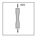
Strain controlled test on smooth specimen
