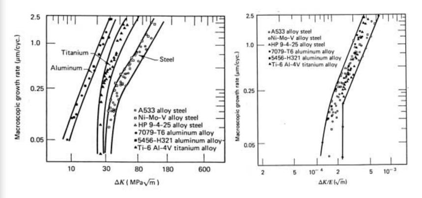
The fatigue crack growth rates for Al and Ti are much more rapid than steel for a given  $\Delta K$ . However, when normalized by Young's Modulus all metals exhibit about the same behavior.
