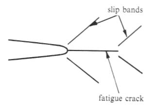
Stage II crack growth (rc >> d)
